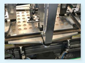
HORIZONTAL CREASING Creasing clamps allow clean carton folds without usage of blades.
